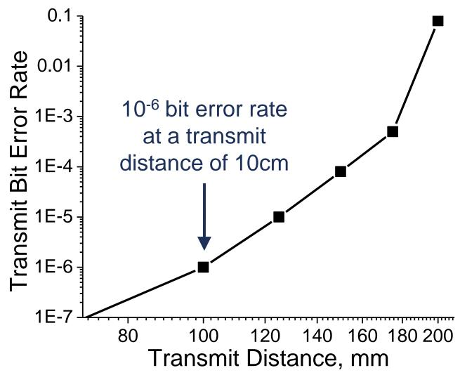
Transmit media is 0.5 mm saline and air to represent the aqueous humor and distance between eye and external device
