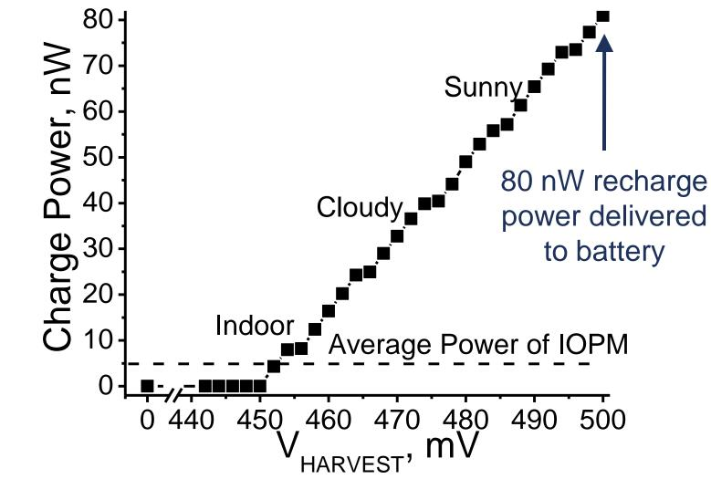
Energy autonomous operation with 1.5 hours of sunlight or 10 hours of indoor lighting per day
