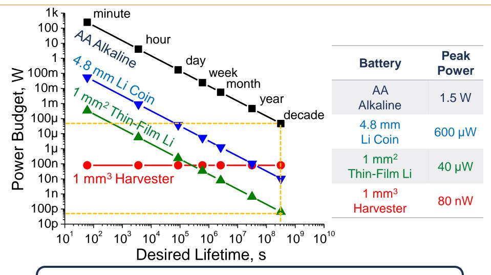
Microsystem volume constraints heavily limit power source capabilities and load circuit power consumption
